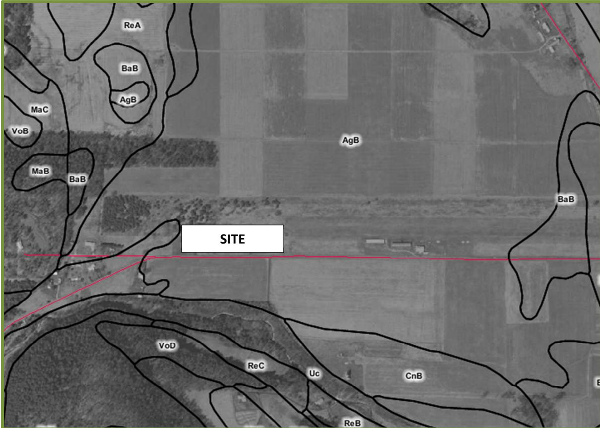
Figure 1. Soil Identification Map for Northeastern Pennsylvania Office Building
